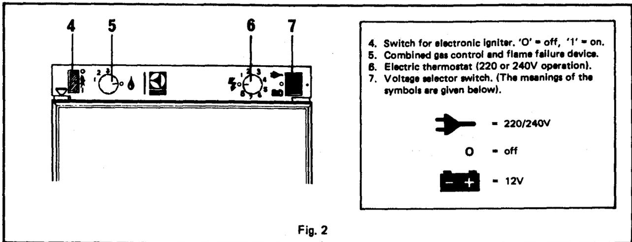
3. Turn the knob (5) of the gas control valve so that the indicator mark is opposite setting No.3.
