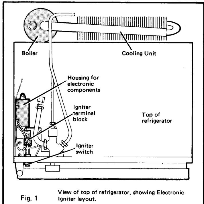
**Fig. 1****View of top of refrigerator, showing Electronic Igniter layout.**
